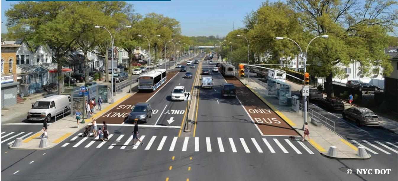
times and increasing ridership capacity. BRT cuts travel time by offering riders the option of paying before they board the bus, traveling in dedicated bus lanes with transit signal priority to reduce the time that buses sit at red lights. BRT has been implemented in cities around the world.
