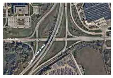
Cyclists crossing the 103rd Street interchange east-west, even on a sidepath, would be required to cross 4 potential points of conflict in each direction as they pass vehicle on/off ramps.
